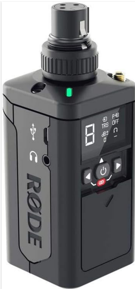
Figure 1.1: Front view of the Rode RodeLink TX-XLR Wireless Plug-On XLR Transmitter, showcasing its compact design and XLR connector.
