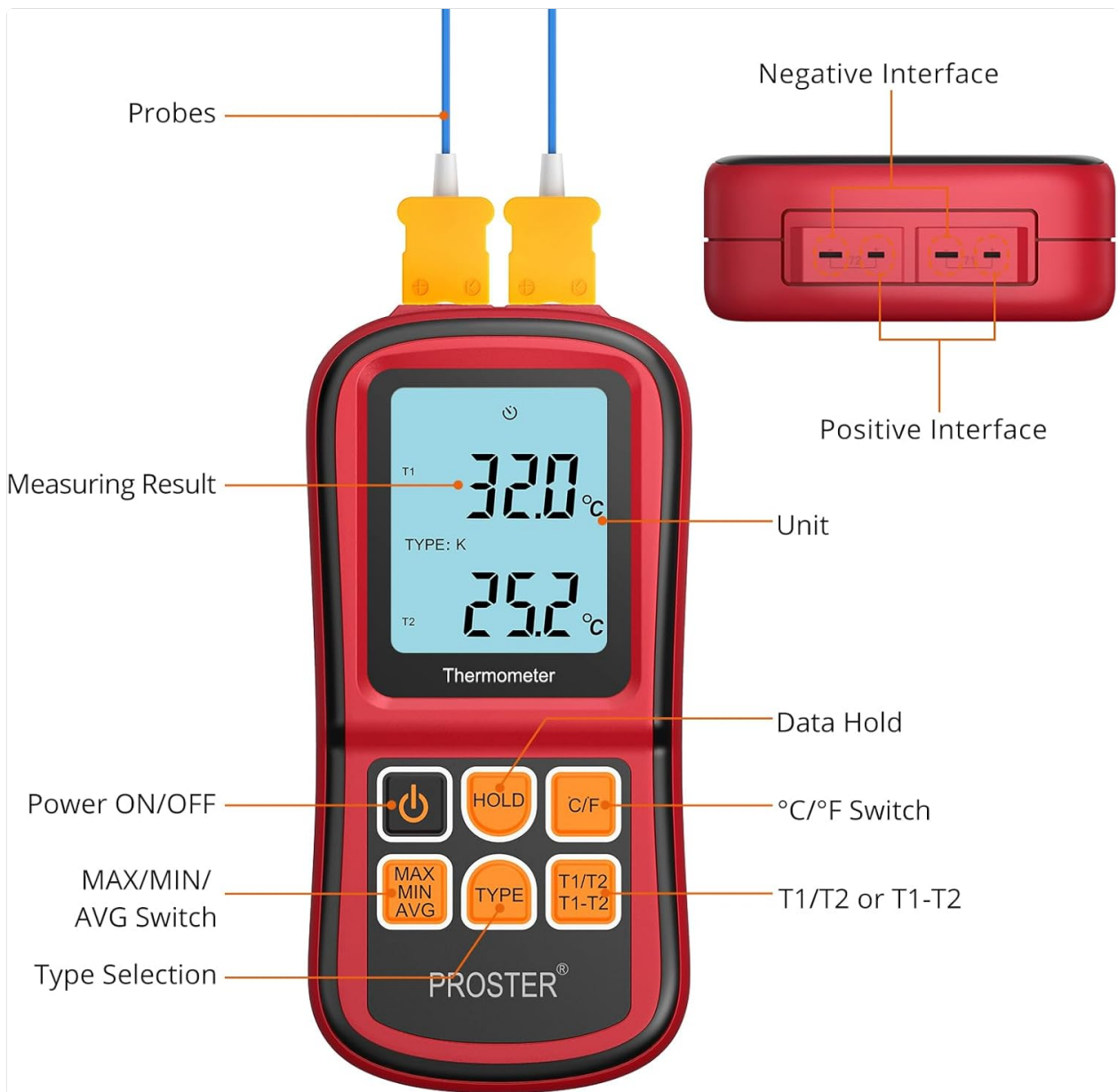
Figure 4.2: Thermometer Components and Controls
