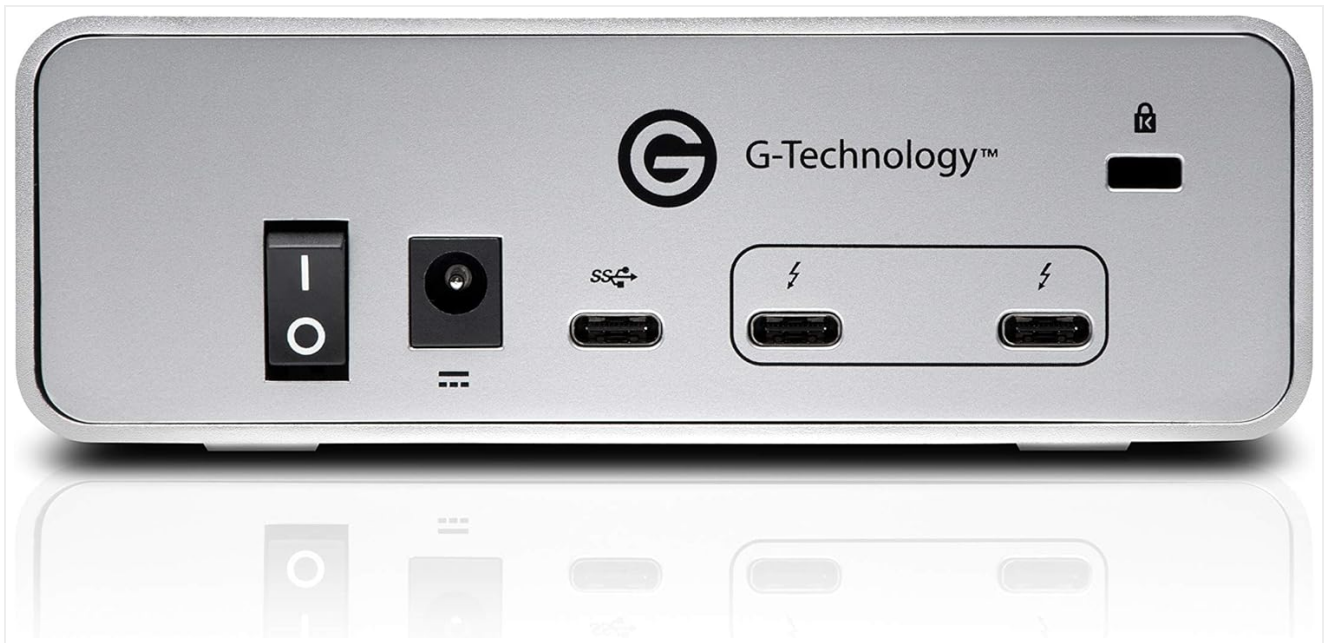
Figure 1: Rear ports of the G-DRIVE, including the power input, USB-C, and dual Thunderbolt 3 ports.
