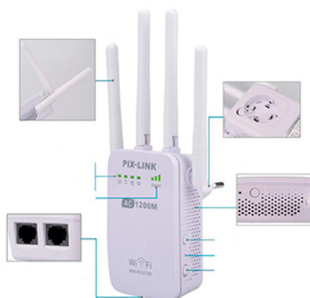
Image: Diagram highlighting key features of the PIX-LINK AC1200, including the four external antennas, power plug, ventilation holes, and Ethernet ports.
