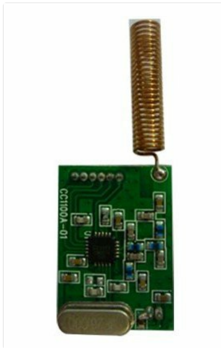
Figure 1: CC1101TR4S Wireless Transceiver Module. This image shows the compact module with its pin headers, ready for integration into a circuit board.
