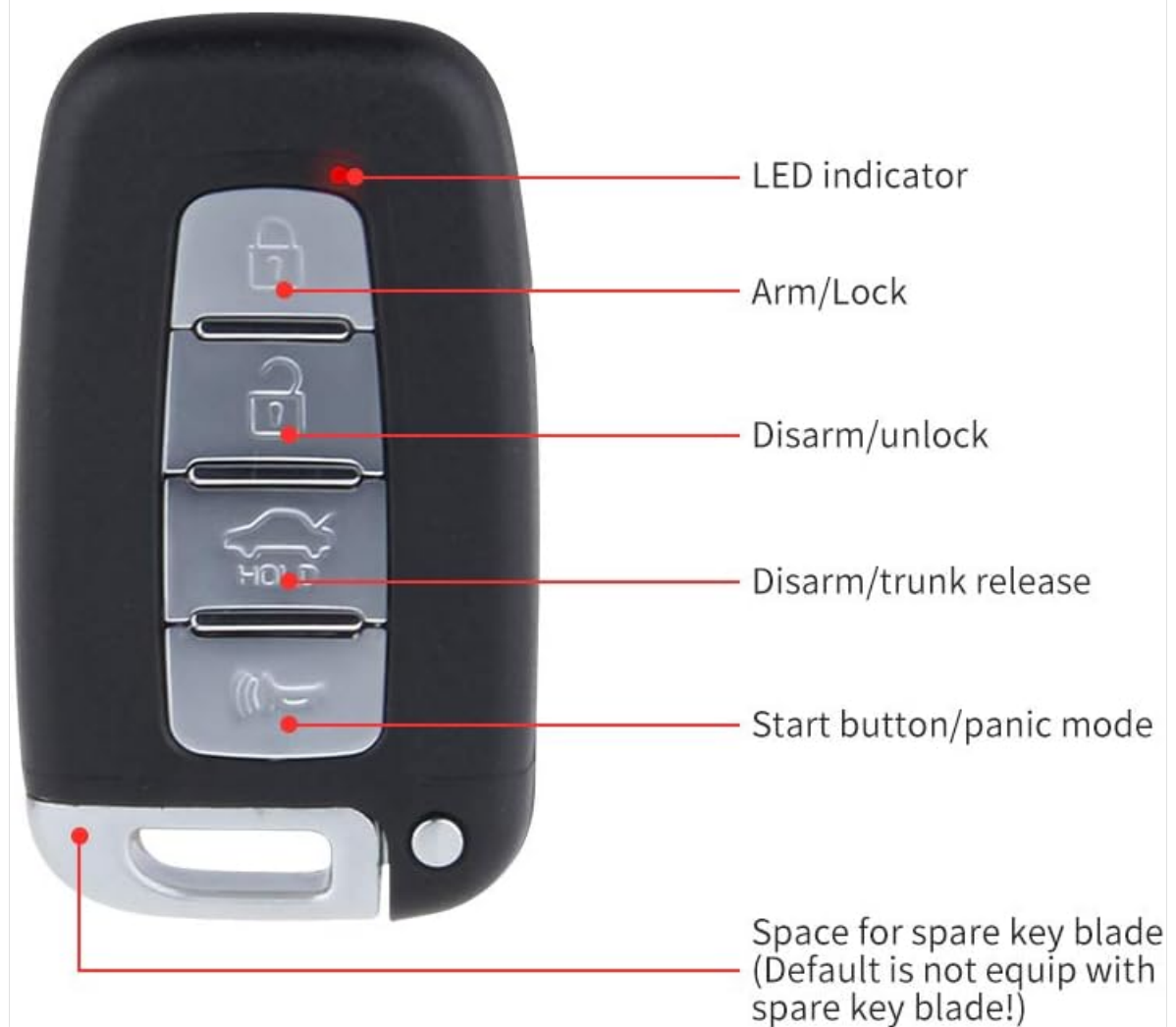
Figure 2.3: Key fob illustrating LED indicator, Arm/Lock, Disarm/Unlock, Disarm/Trunk Release, and Start Button/Panic Mode functions.
