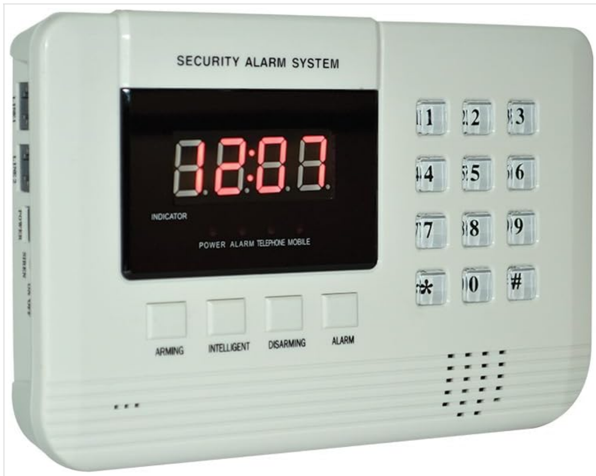
Figure 2.3: Front view of the PNI PG200 main control panel, featuring an LCD display, numeric keypad, and function buttons for arming, disarming, and intelligent modes.
