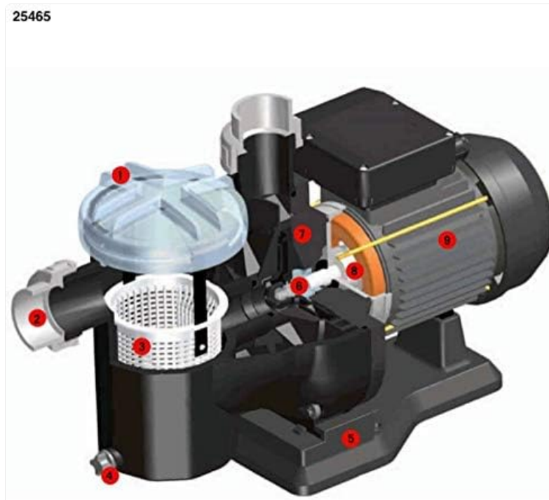
Figure 2: Exploded view of the Astral Sena pump components. This diagram illustrates the internal structure, including the pre-filter basket (1), suction connection (2), drain plug (4), pump base (5), mechanical seal (7), impeller (8), and motor (9).
