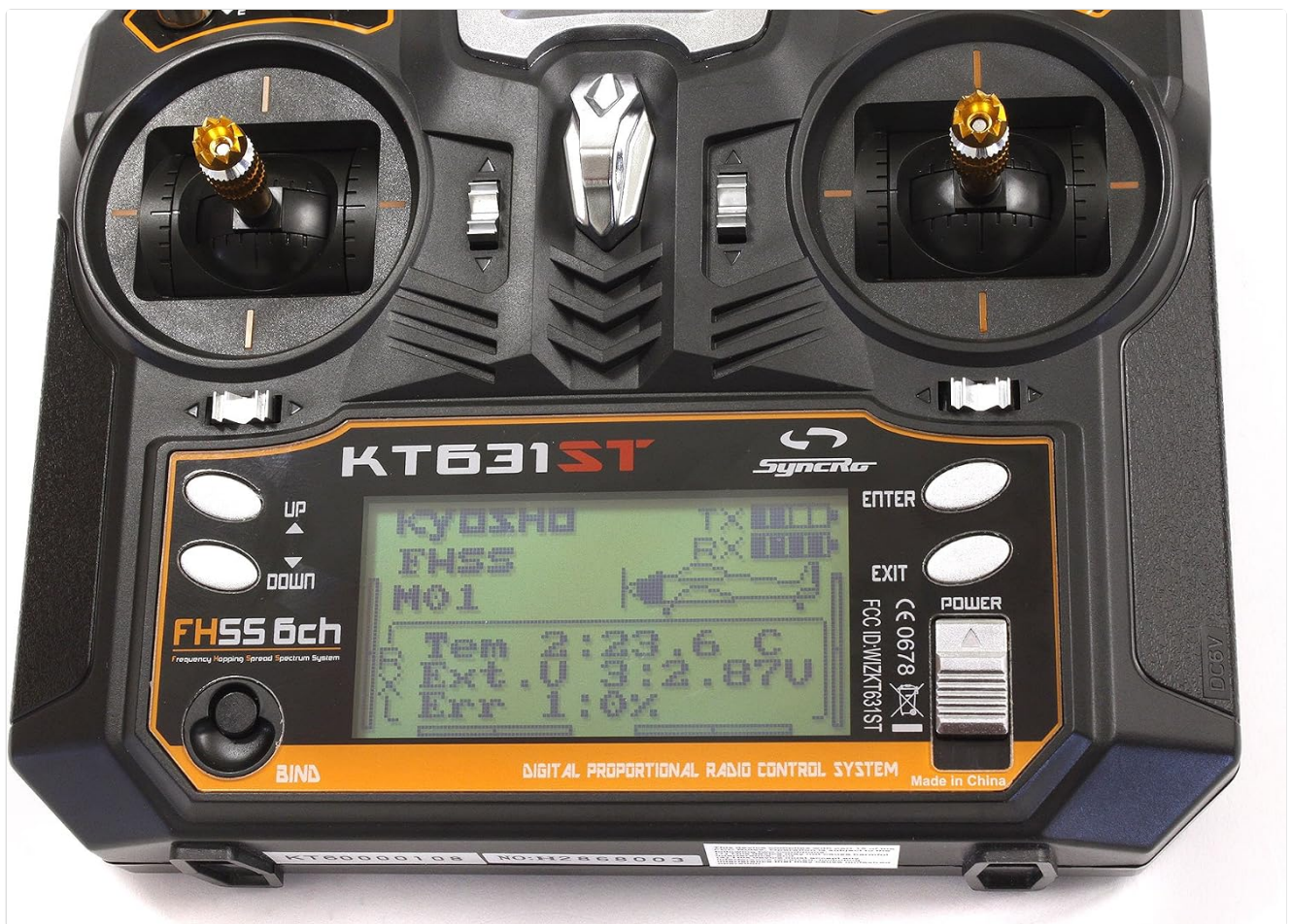
Figure 4: Close-up view of the KT-631ST transmitter's LCD screen, showing telemetry data such as temperature, external voltage, and error rate.
