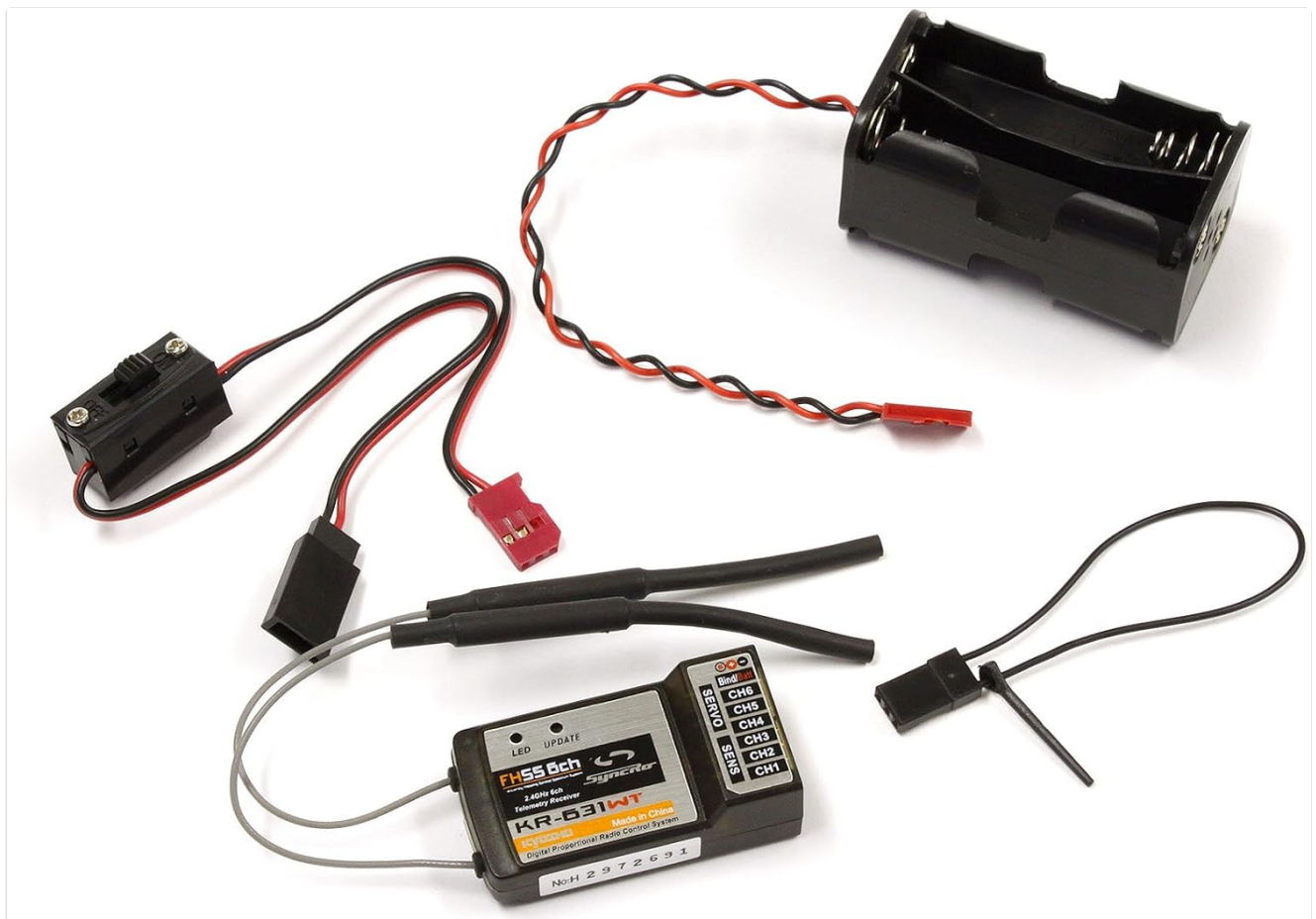
Figure 5: The Kyosho KR-631WT receiver with its dual antennas, binding plug, and battery holder, ready for installation.
