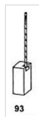
Figure 2: Illustrative diagram of a carbon brush assembly, similar to the component being installed.
