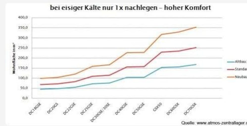
Image 5.1: Refueling Frequency - 1x per day for high comfort in very cold conditions. This chart shows the heated living area (Wohnfläche in m 2 ) on the Y-axis against different ATMOS boiler models on the X-axis, with three lines representing old buildings, standard buildings, and new buildings, indicating the area that can be heated with one refueling per day.
