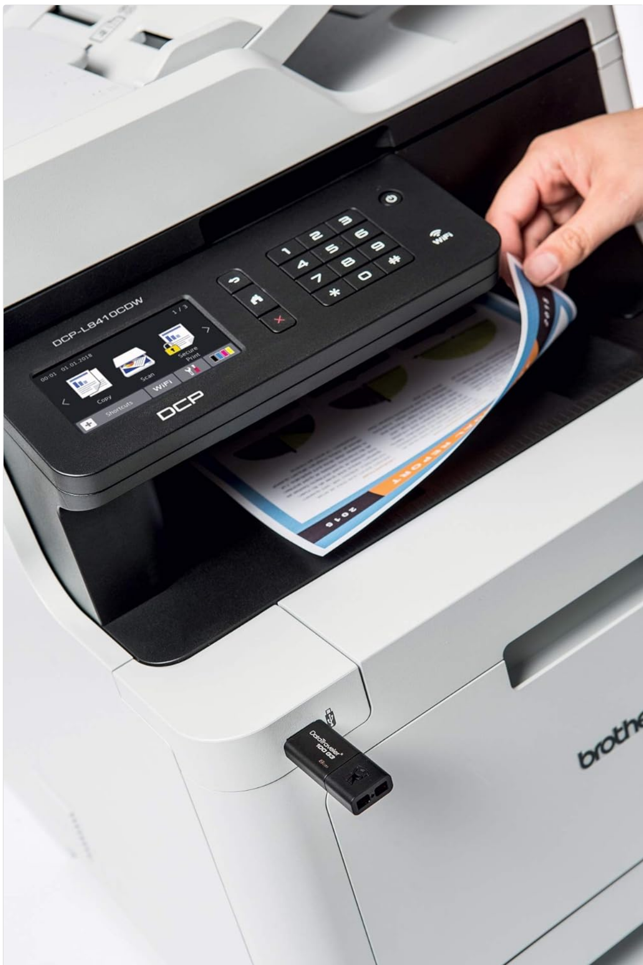
Image 3.2: Using the Automatic Document Feeder for scanning or copying, and the USB port for direct printing/scanning.
