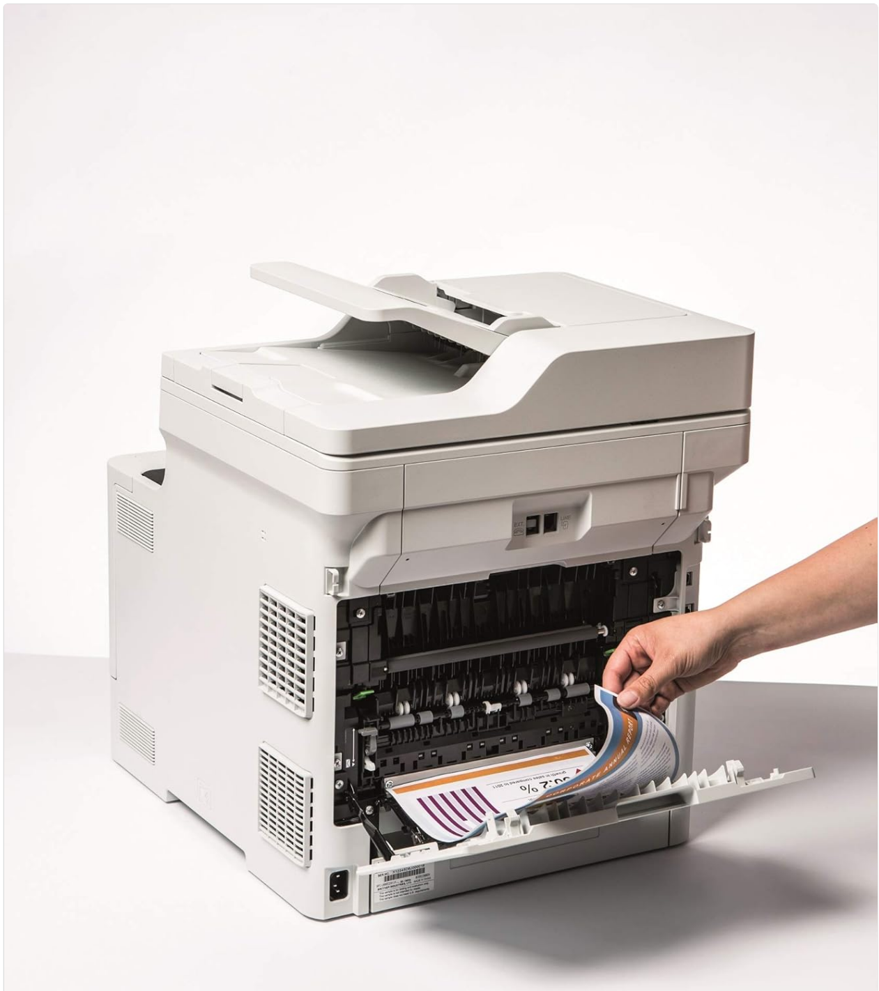
Image 5.1: Clearing a paper jam from the rear of the printer.
