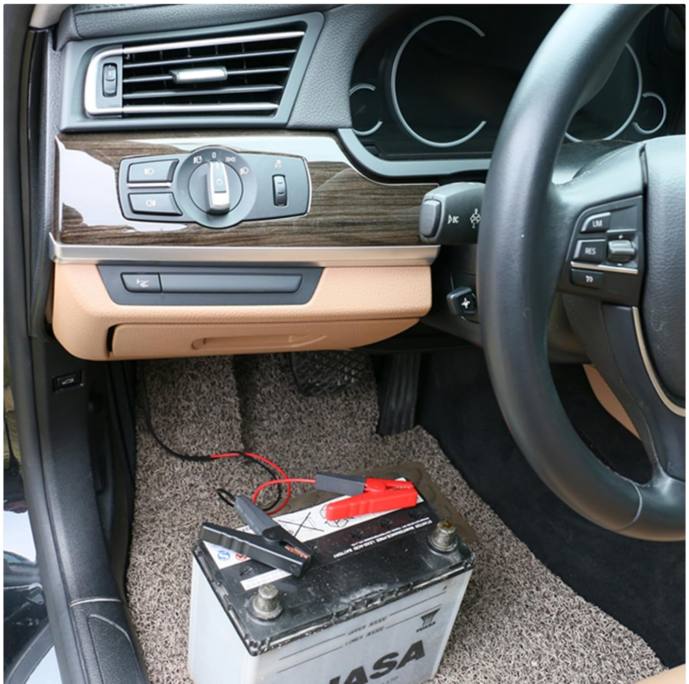
Figure 3: An in-car perspective showing the BT30 connected to the OBD-II port, with the external battery placed on the floor.
