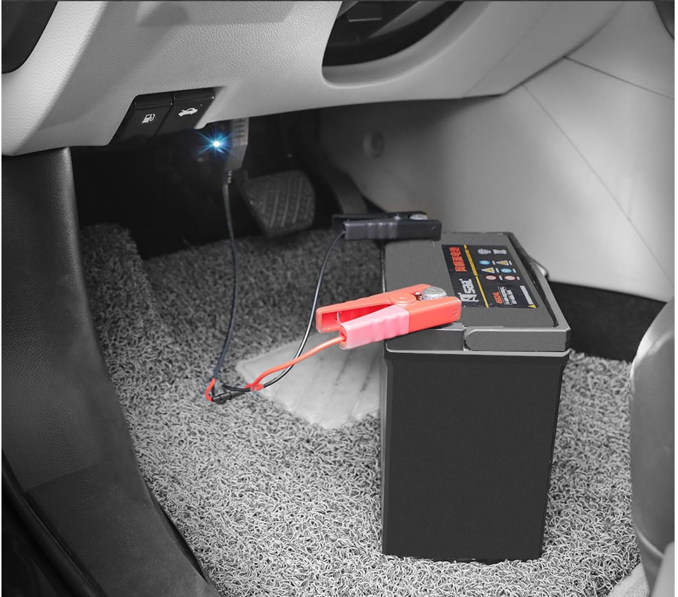
Figure 2: The BT30 tool connected to the vehicle's OBD-II port and an external 12V battery, providing continuous power.
