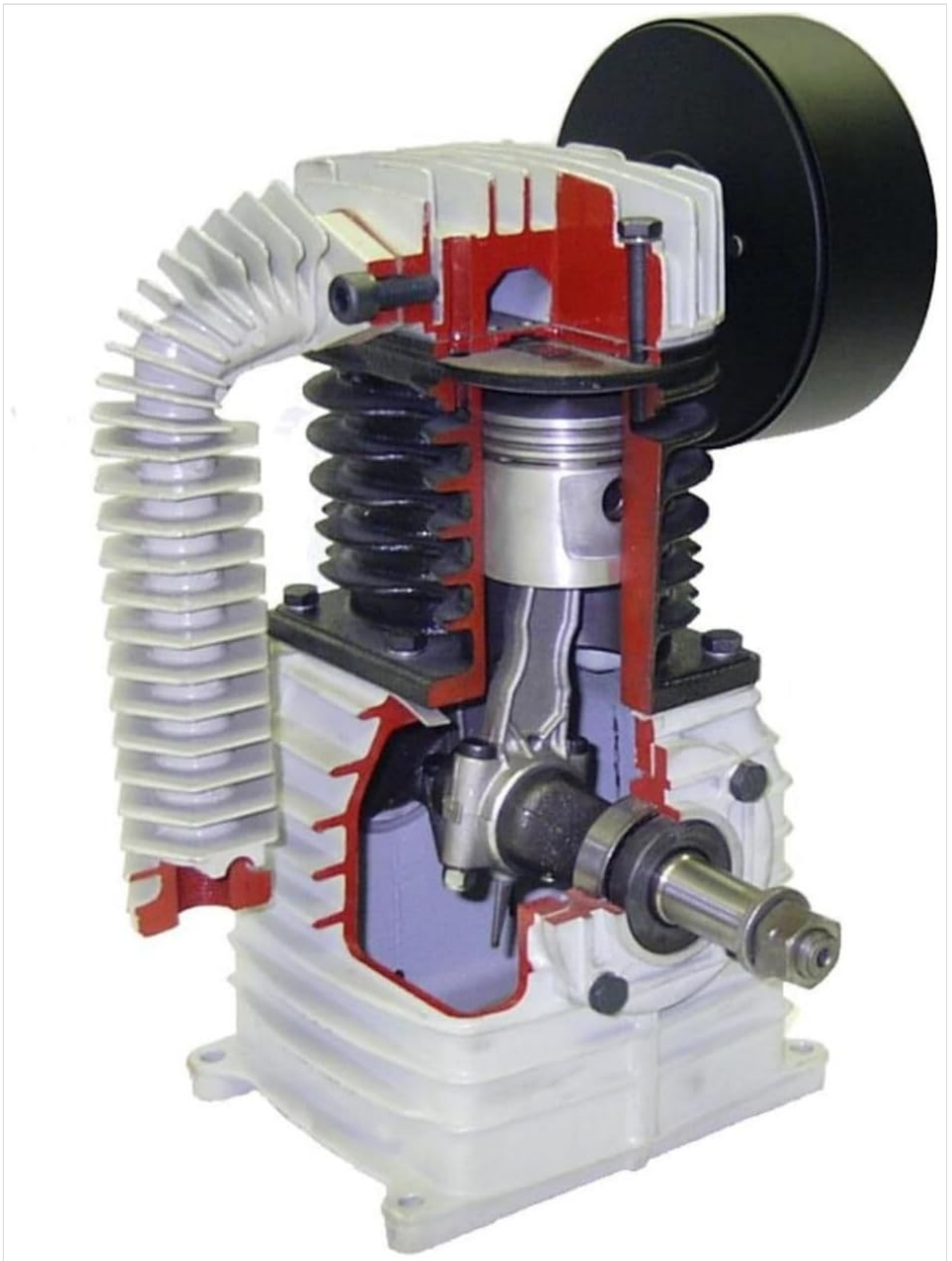
Figure 2: Cutaway view of the Rolair air compressor pump. This image illustrates the internal components of the pump, including the piston, connecting rod, and crankshaft, highlighting the double-cylinder, single-stage design.
