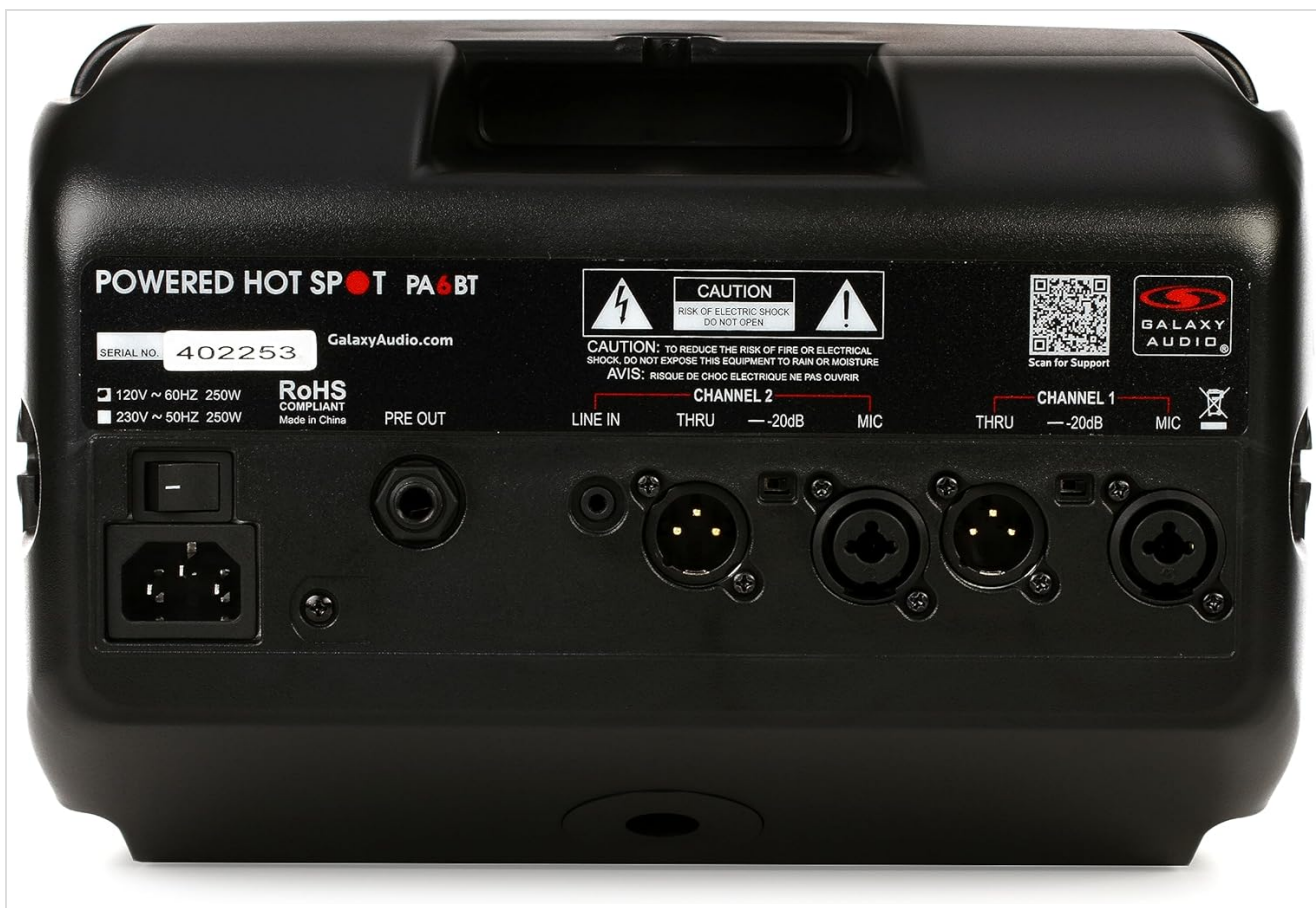
Figure 3: Rear view of the Galaxy Audio PA6BT monitor, displaying the power input, serial number, and various audio input/output connections for Channel 1 and Channel 2.
