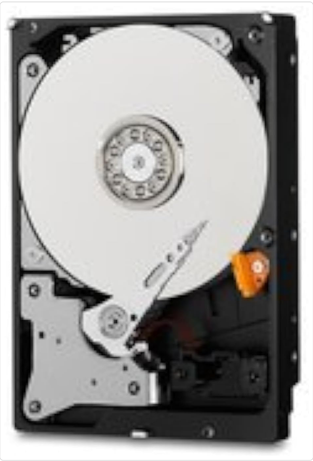
Image 2: Internal components of a hard disk drive, illustrating the mechanical nature of the storage.
