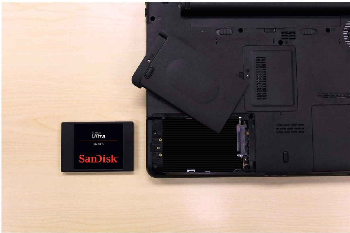
Figure 5: SanDisk Ultra 3D SSD ready for installation into a drive bay or external enclosure.
