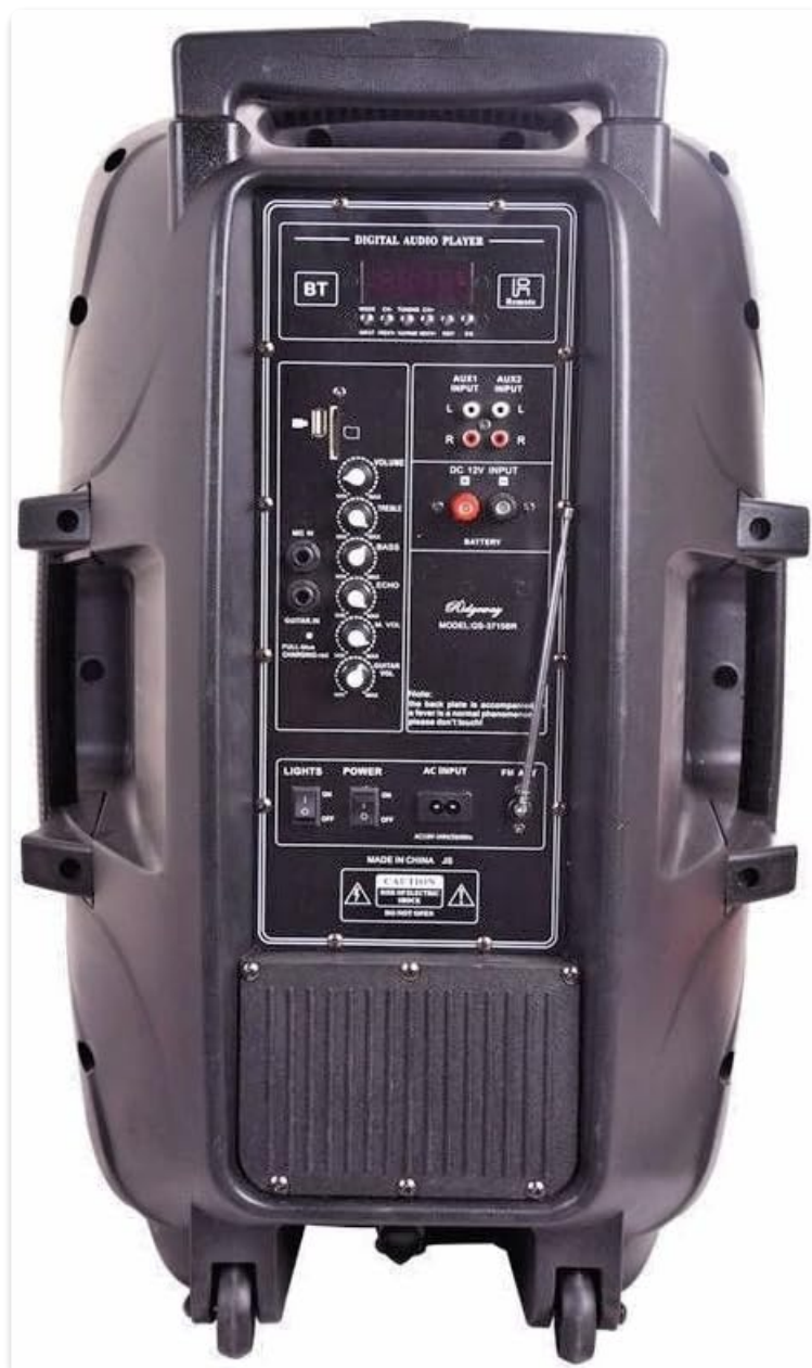
Figure 2: Rear view of the speaker, highlighting the control panel with various inputs (USB, SD, Aux, Mic), volume controls, and power connections.
