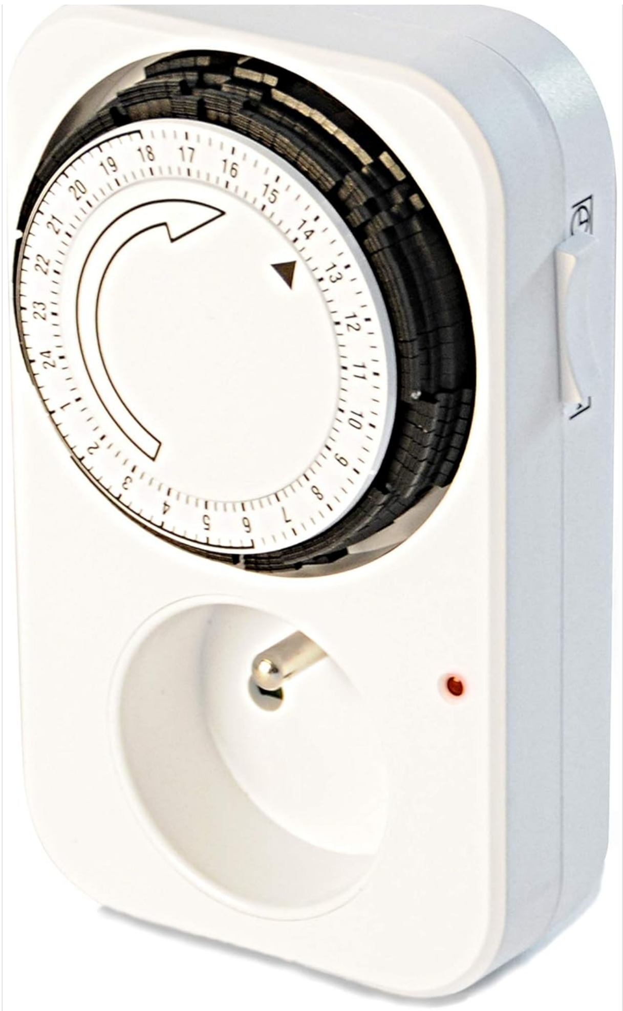
Figure 1: Front view of the SCS Sentinel MecaProg INDOOR Mechanical Programmable Timer Plug. This image shows the main dial with numbers 1-24 representing hours, and the pins around the dial for setting 15-minute intervals. The
