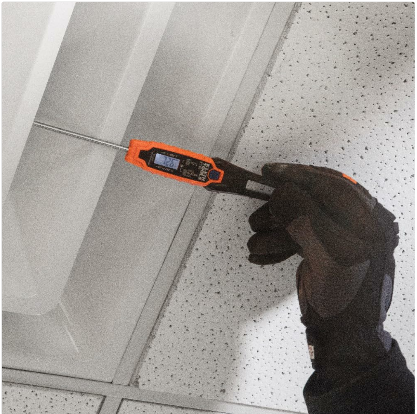
Image: The Klein Tools ET05 thermometer being used to measure the temperature inside an HVAC vent.
