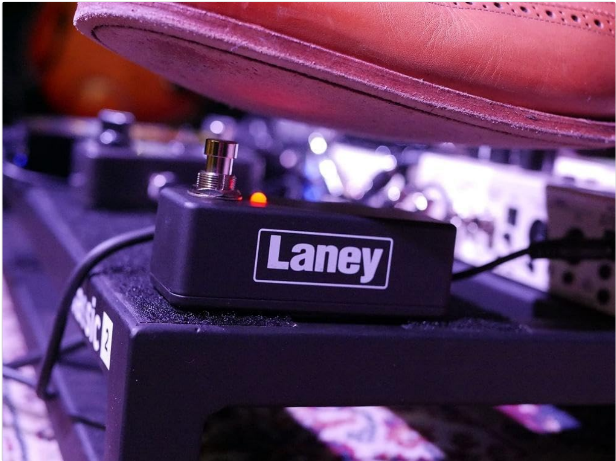
Image: The Laney FS1-MINI footswitch positioned on a pedalboard, with a foot about to engage the switch. The red LED is illuminated, indicating its operational status.
