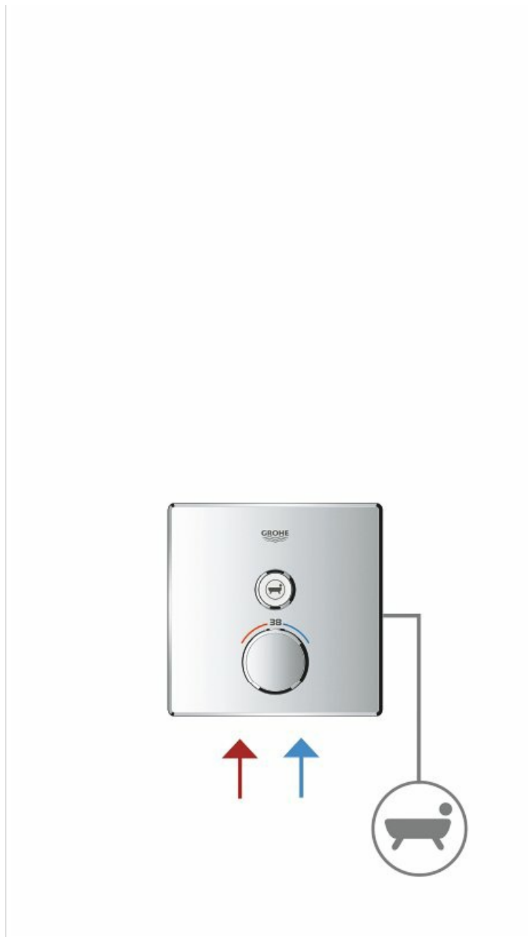
Image 4.3: Diagram illustrating a plumbing configuration for the Grohtherm SmartControl system with a single water outlet, such as a shower head or bathtub filler. Red and blue arrows indicate hot and cold water inlets.
