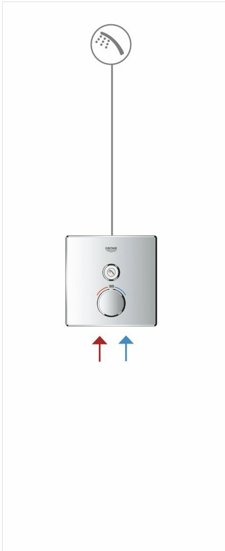
Image 4.2: Diagram illustrating potential plumbing configurations for the Grohtherm SmartControl system with multiple water outlets (e.g., hand shower, overhead shower, side jets). Red and blue arrows indicate hot and cold water inlets.
