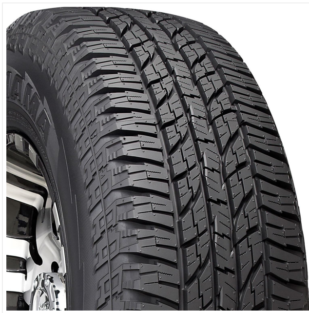
Image 4.1: A detailed view of the Yokohama Geolander A/T G015 tread pattern, highlighting its sipes and grooves.
