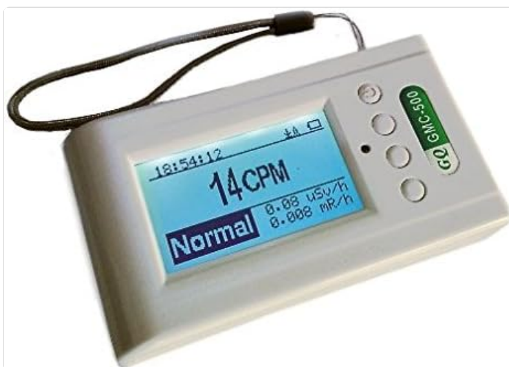
Figure 4.2: Angled view of the GQ GMC-500, highlighting its compact design and the arrangement of the display and side buttons. The screen shows 14 CPM and a "Normal" radiation level.
