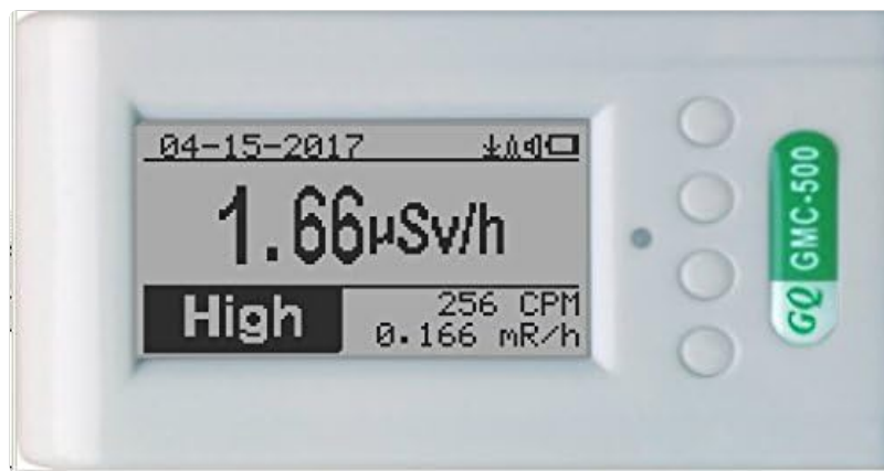
Figure 4.3: Close-up of the display showing a "Normal" radiation reading of 1.66 \mu\text{Sv/h} , 256 CPM, and 0.166 mR/h.
