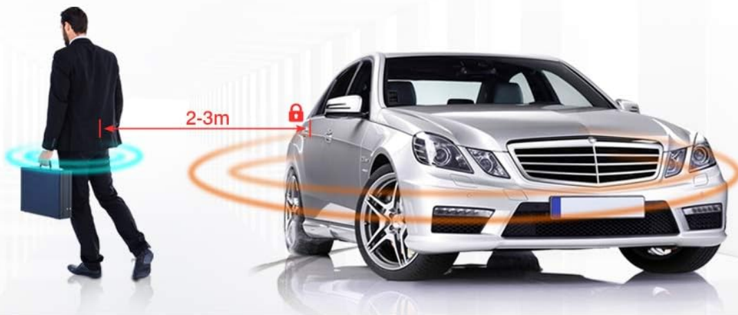
Figure 5.1: PKE Passive Keyless Entry operation.
