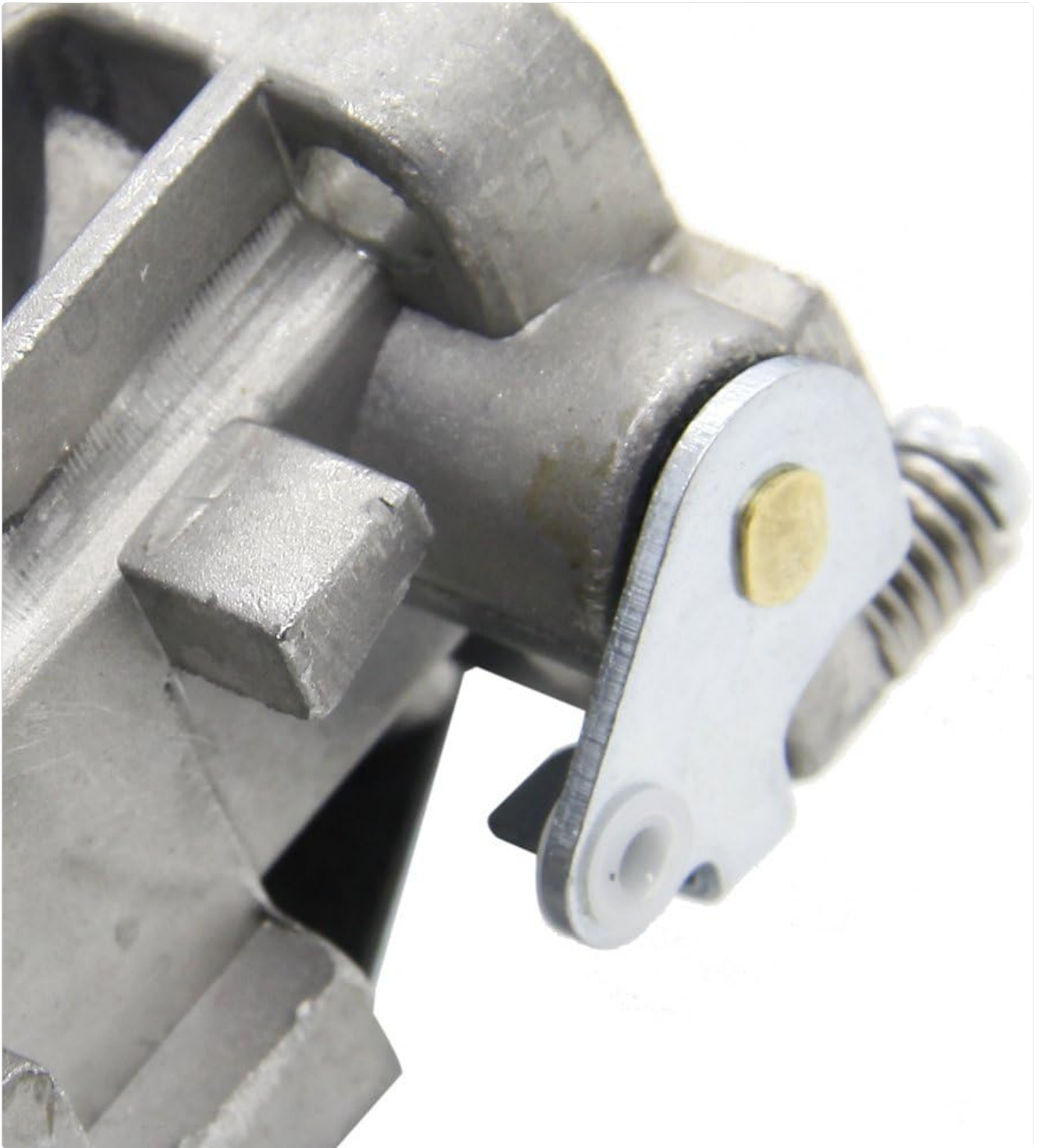
Figure 3: Detail of the throttle linkage spring mechanism on the carburetor. Note the position and connection points of all springs and rods before removal.
