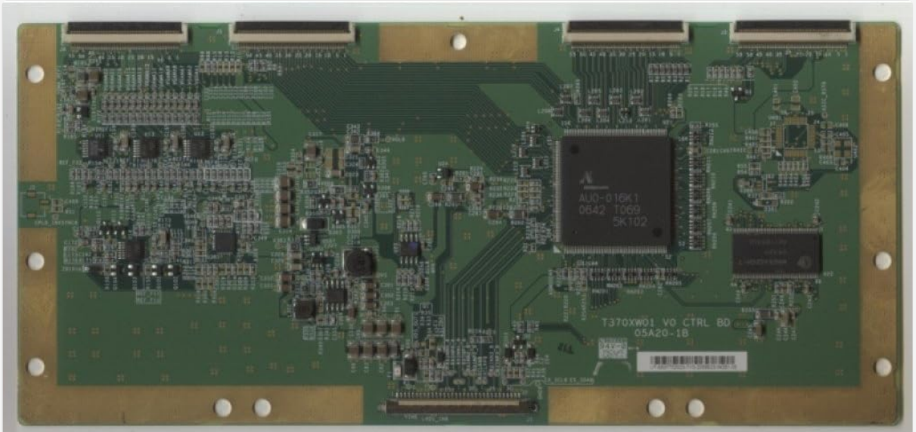
Figure 1: T370XW01 V0 CTRL BD 05A20-1B T-Con Board. This image displays the T370XW01 V0 CTRL BD 05A20-1B T-Con board, a green circuit board with various integrated circuits, capacitors, resistors, and connectors. The board features a large central chip labeled 'AUO-016K1' and multiple ribbon cable connectors along the top and bottom edges. The overall design is rectangular with mounting holes at the corners.
