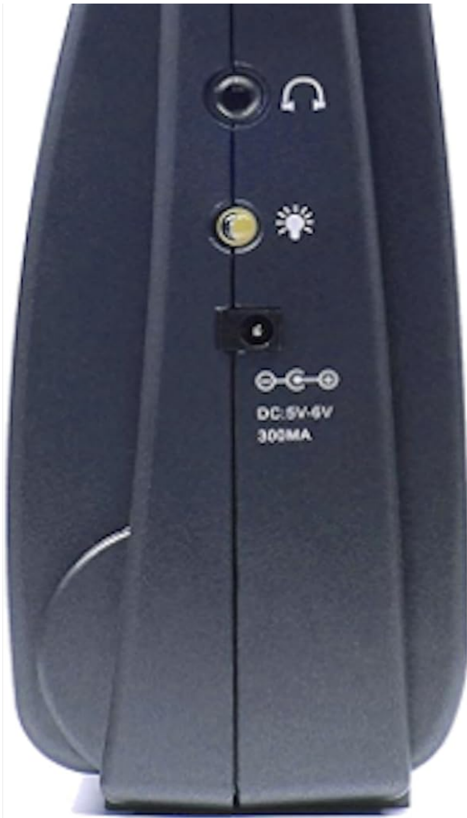
Figure 3: Left side view of the Kaito KA390, showing the DC power input, flashlight switch, and earphone jack.
