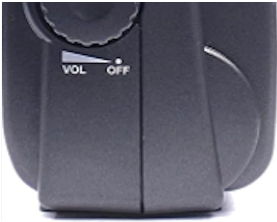
Figure 5: Right side view of the Kaito KA390, illustrating the combined volume and power knob.
