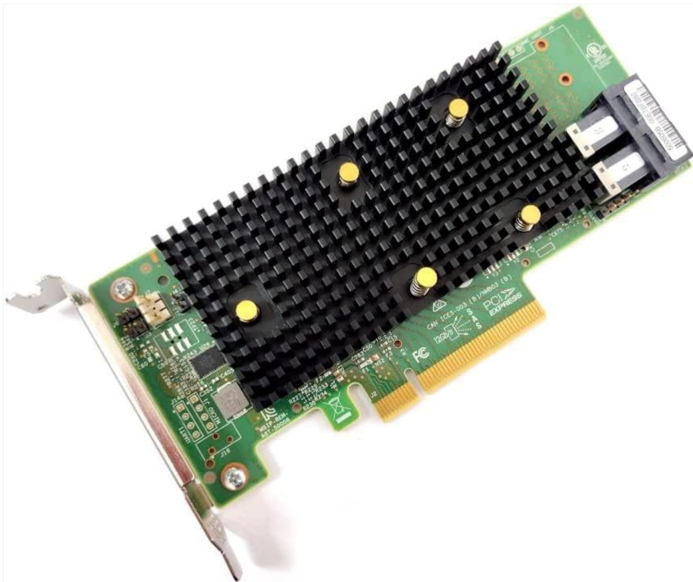
Figure 2.2: Top view of the MegaRAID 9440-8i controller, displaying the large heatsink for thermal management and the two SFF-8643 Mini-SAS HD connectors.
