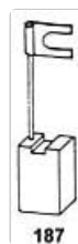
Figure 2: A schematic diagram illustrating the structure of a carbon brush, including the carbon block and its electrical connection. This helps in understanding the component's design for correct installation.
