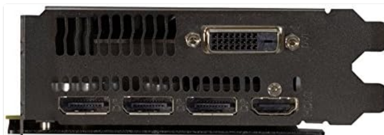
Figure 3: Rear I/O panel of the graphics card, showing the DL DVI-D, HDMI, and DisplayPort outputs for monitor connections.
