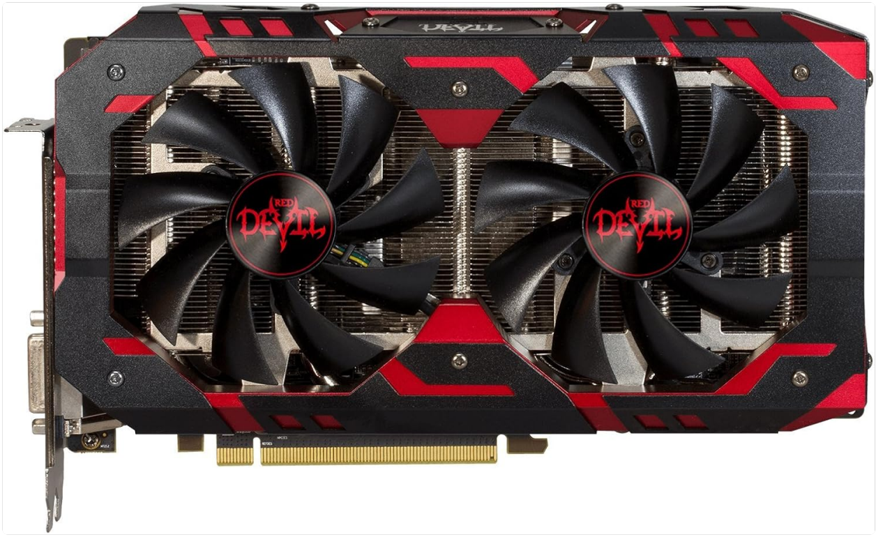
Figure 1: Front view of the PowerColor AMD Radeon RED DEVIL RX 580 Graphics Card, showcasing its dual-fan cooling solution.
