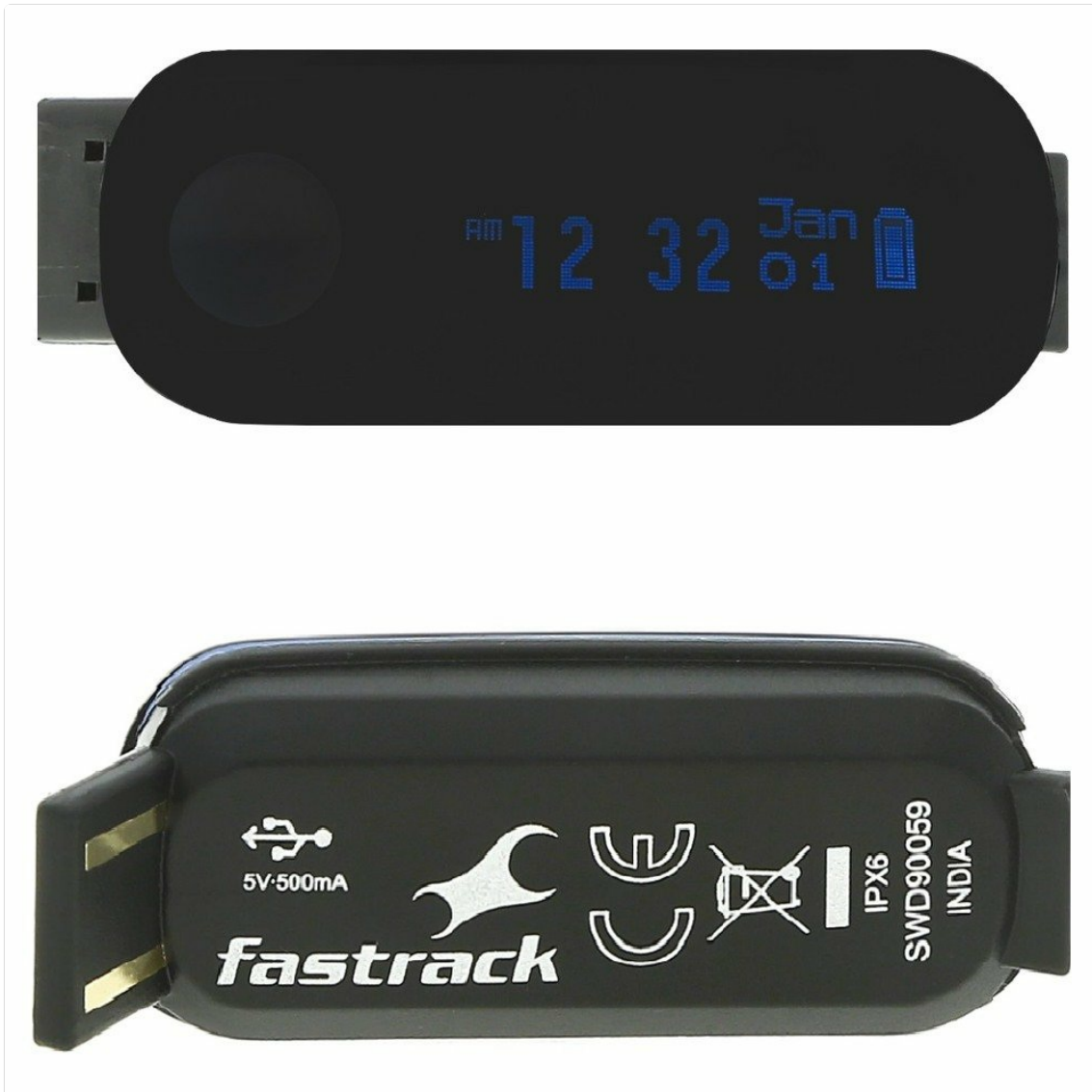
Image 2: The main unit of the Fastrack Reflex Smartwatch Band, showing the integrated USB charging port.
