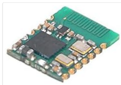
Figure 2: An angled perspective of the module, showcasing the integrated antenna on the right side and various surface-mount components, including the main chip and Murata capacitors.
