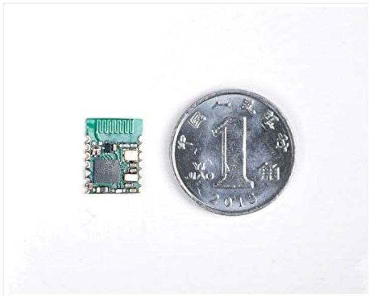
Figure 1: This image shows the compact size of the NRF51822 Bluetooth module, positioned beside a Chinese Yuan coin to illustrate its small dimensions.
