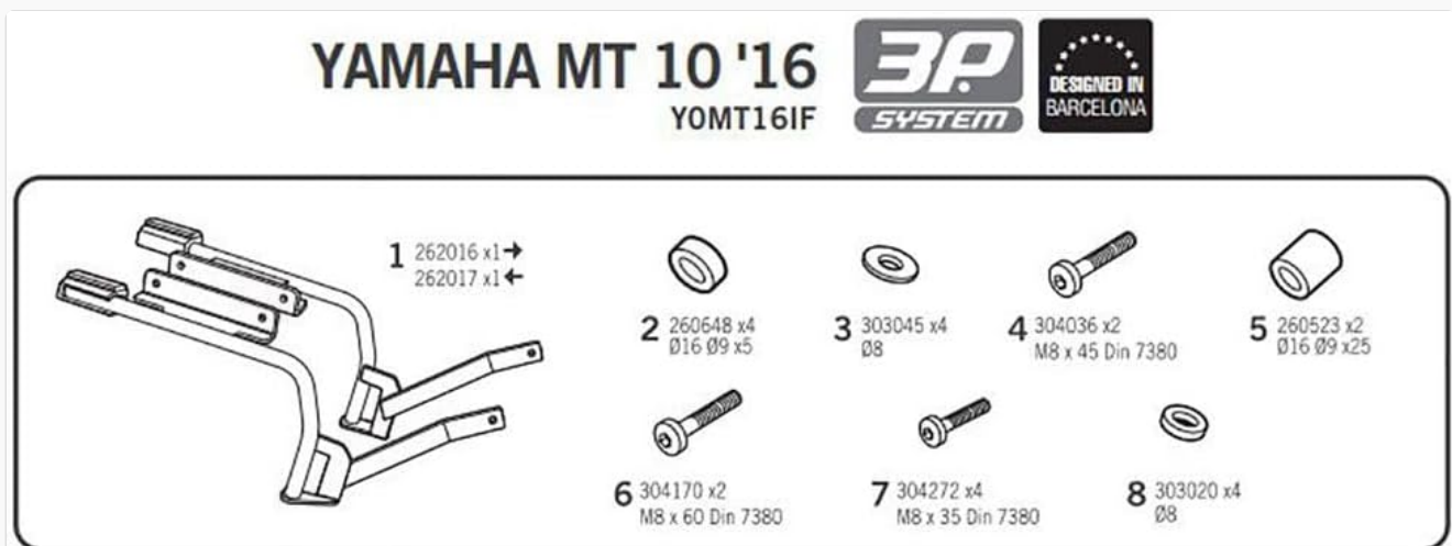
Image 2.1: Exploded view of the SHAD 3P System components and hardware. This diagram illustrates each part of the mounting kit, including bolts, washers, and spacers, with corresponding part numbers and quantities for assembly.
