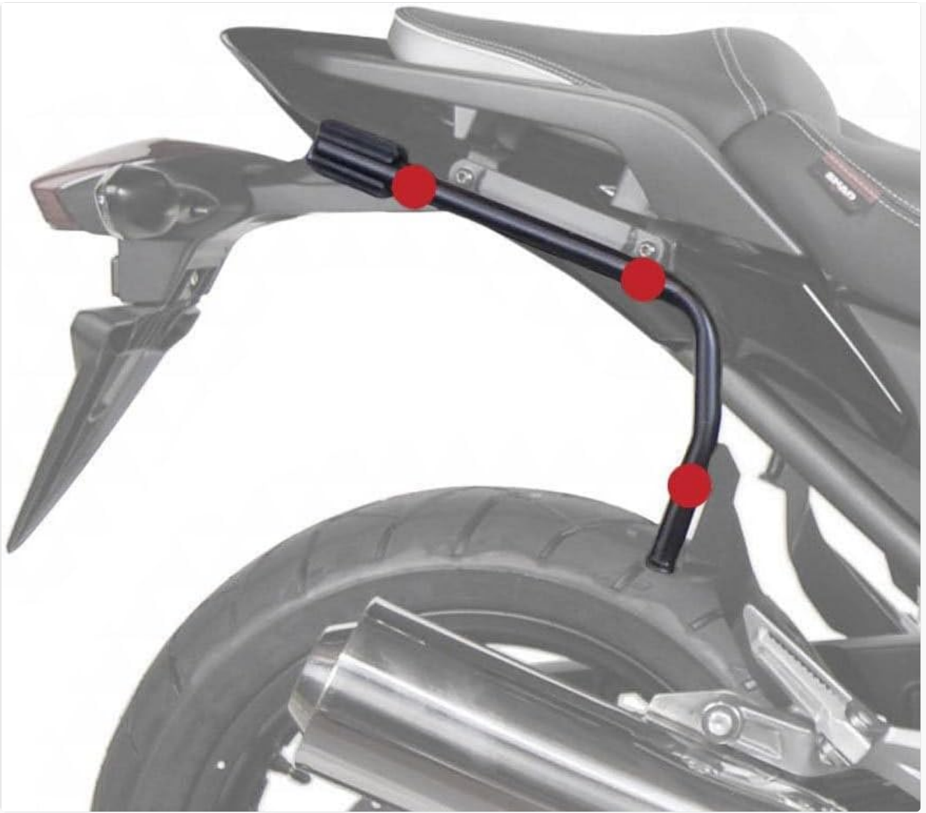
Image 3.2: Close-up view of the SHAD 3P System Side Mount installed on a motorcycle, highlighting the three attachment points with red markers. This illustrates the secure and minimal connection points of the system to the bike's frame.
