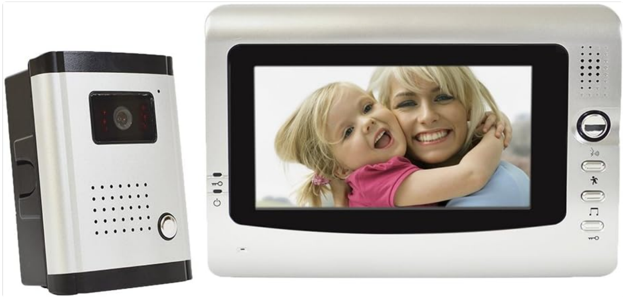
Figure 2: The indoor monitor with its 7-inch LCD screen, showing control buttons on the right side for various functions like monitoring, speaking, and unlocking.
