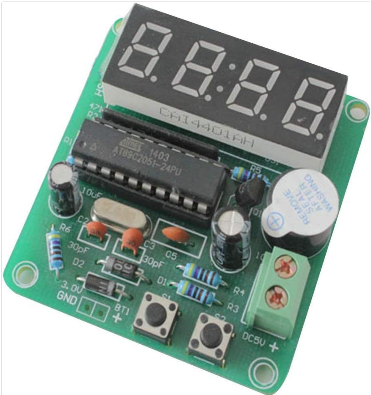
Image 4.1: The fully assembled DAOKI C51 Digital LED Electronic Clock circuit board, showing all components soldered into place and the LED display mounted.
