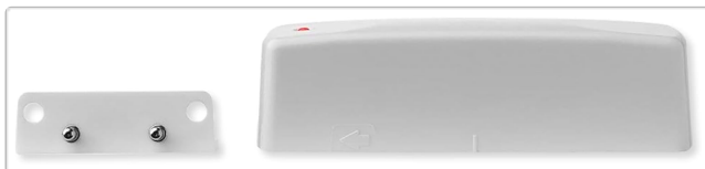
Figure 4.2: The main sensor unit and the separate water probe, highlighting the two metal contacts on the probe for water detection.
