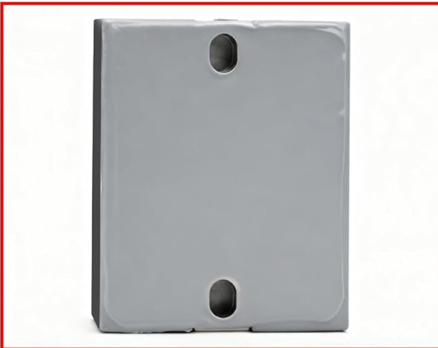
3. Apply thermal grease evenly
