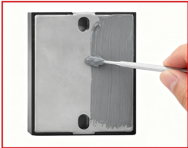
2. Use a brush to spread the thermal grease
