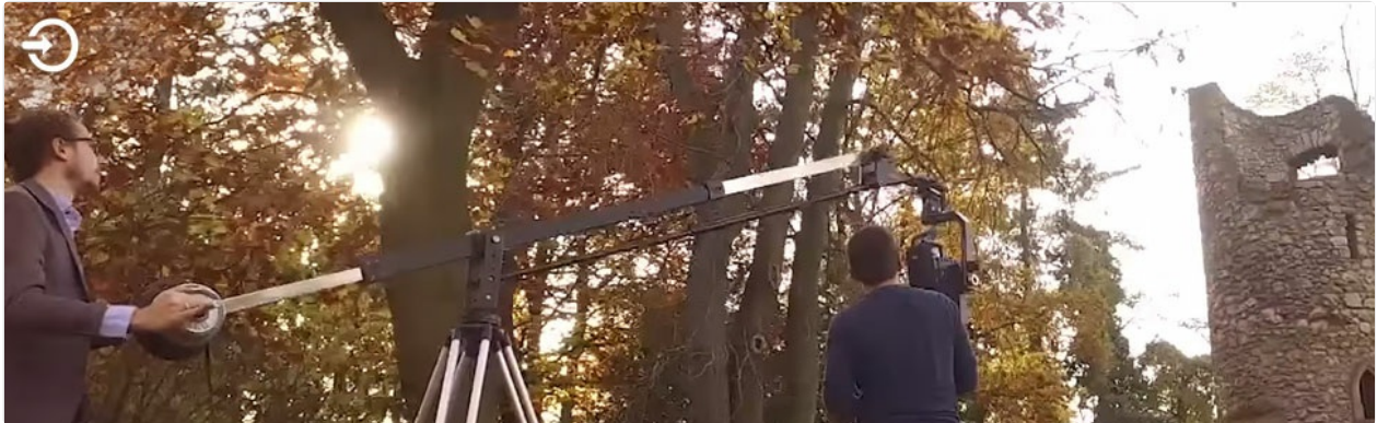
Image: The PROAIM Wave-2 Jib Crane demonstrating its professional and versatile design, adapting to direct camera mounting, gimbals, and pan-tilt heads. Supportive accessories are for demonstration only.
