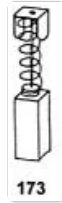
Figure 2: Schematic representation of a carbon brush assembly, illustrating the carbon block, spring, and electrical connection. This diagram aids in understanding the components during replacement.
