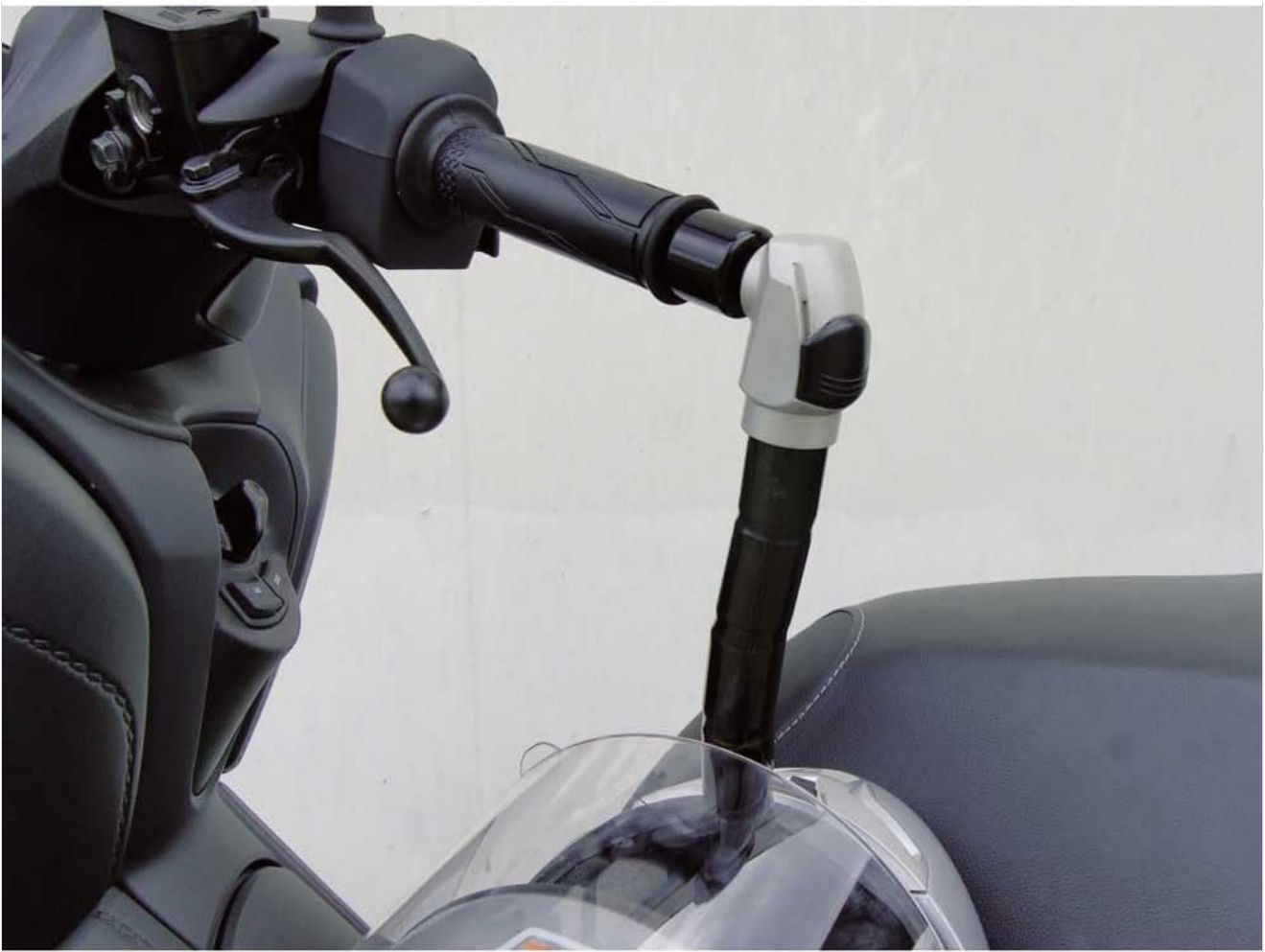
Image: The Artago 778STY handlebar lock stored in its dedicated mounting bracket when not in use, positioned near the scooter seat.
