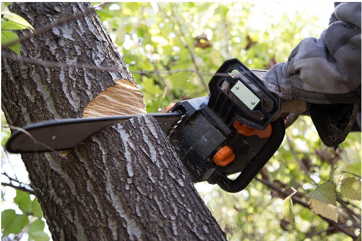
Figure 3: Chainsaw in operation, demonstrating proper two-hand grip and cutting posture.
