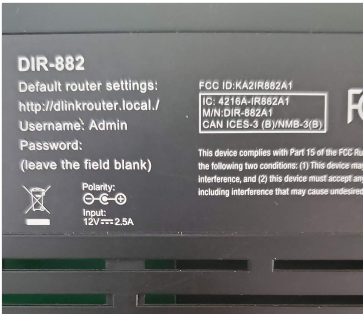
Figure 3: Close-up of the router's bottom label, indicating default router settings: http://dlinkrouter.local./ , Username: Admin, Password: (leave the field blank).
