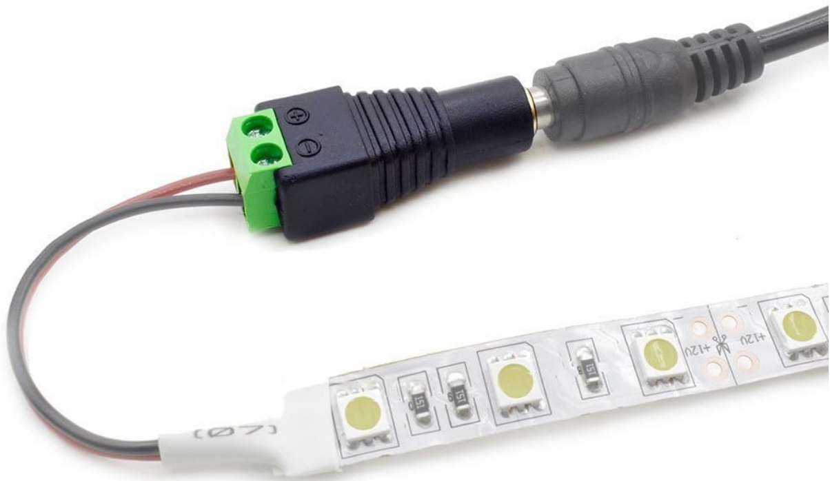
Image 5.2: A close-up view of the DC screw terminal connector properly attached to an LED strip, ready for connection to the power supply.
