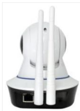
Figure 2.4: Rear view of the NTC V380 camera, highlighting the dual antennas for enhanced WiFi reception and the Ethernet port for wired connection.
