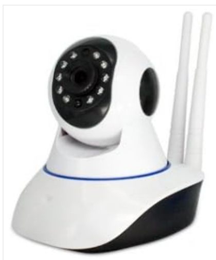
Figure 2.1: Front view of the NTC V380 WiFi Smart Camera, showing the lens, infrared LEDs, and microphone.
