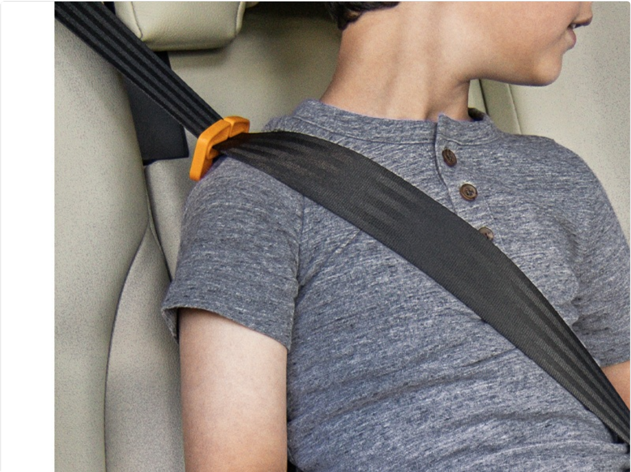
Figure 2: Proper shoulder belt positioning using the shoulder belt clip. The image shows a child in the booster seat with the vehicle's shoulder belt correctly positioned across their shoulder, guided by the orange clip.
