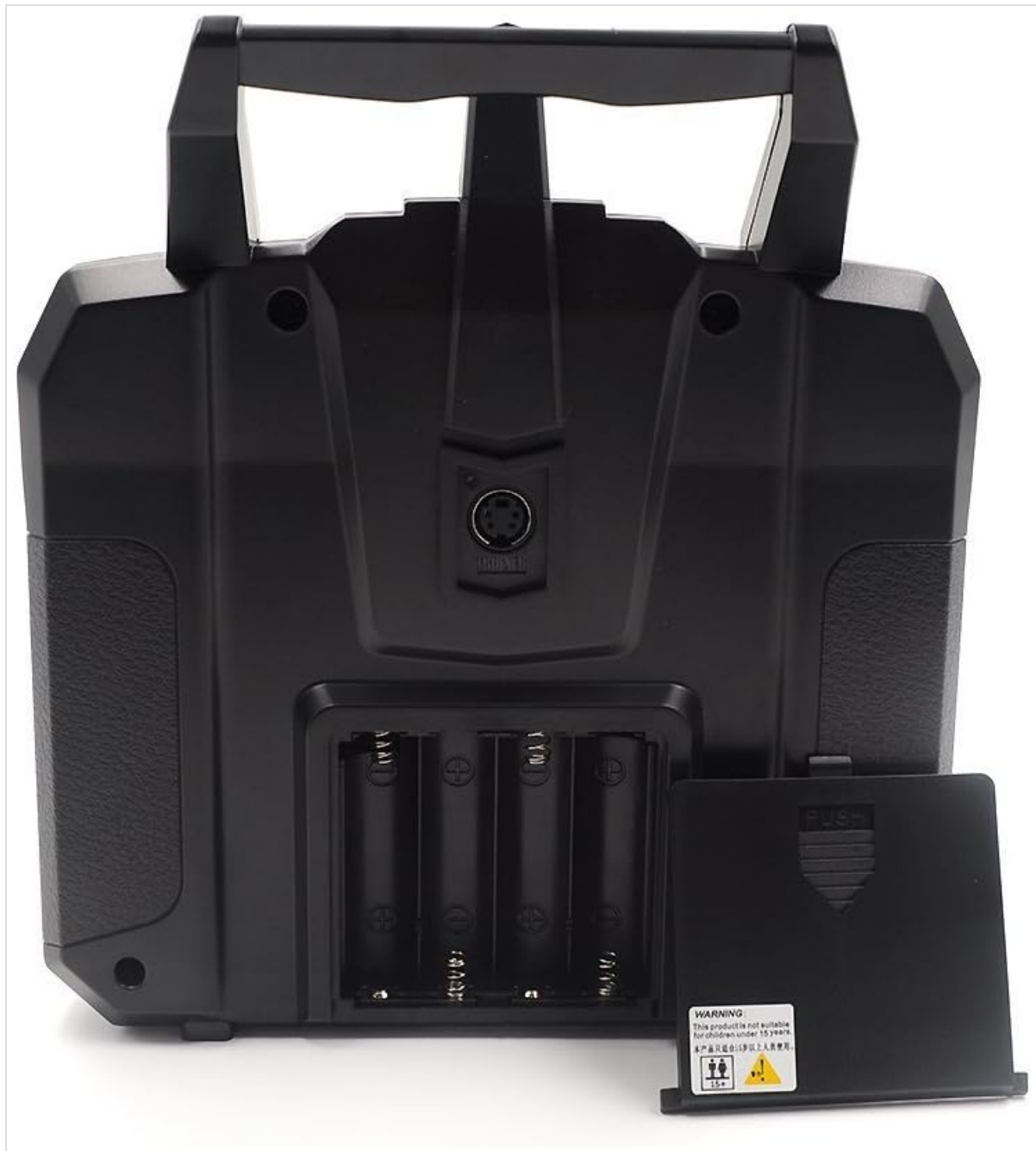
Figure 4.1: Rear view of the FS-i6X Transmitter showing the battery compartment.
