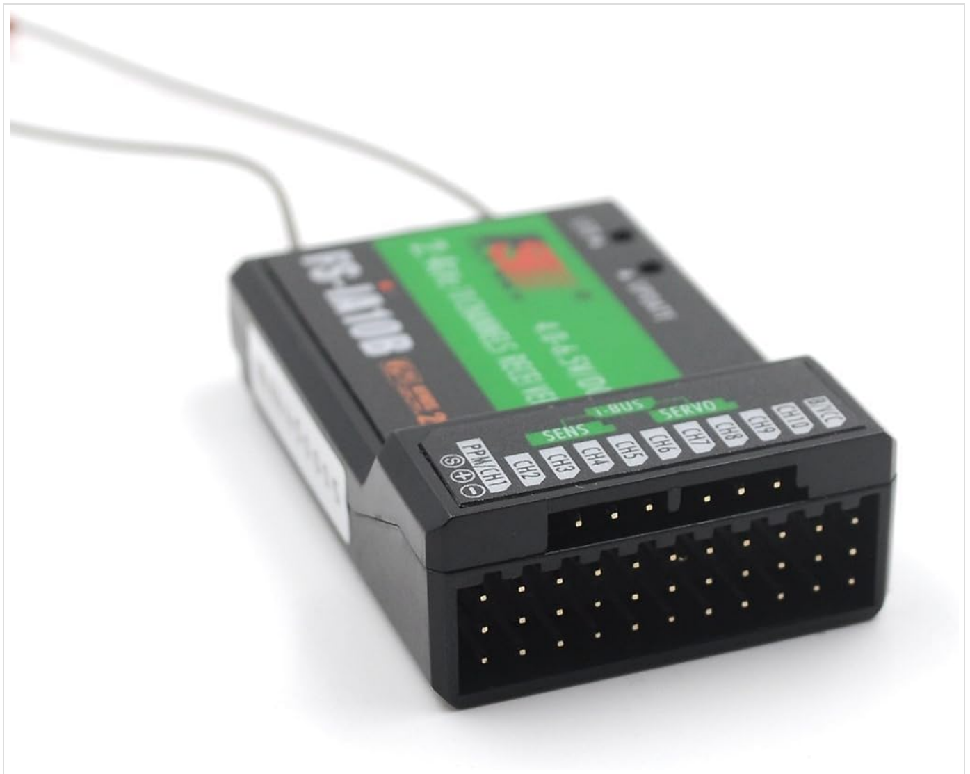
Figure 3.3: Close-up view of the FS-iA10B Receiver showing servo ports and antenna.
