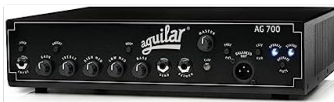
Another perspective of the Aguilar AG 700 bass amplifier head's front panel, highlighting the layout of the input, gain, EQ section (Treble, High Mid, Low Mid, Bass), Deep and Bright switches, and the Master volume control.
