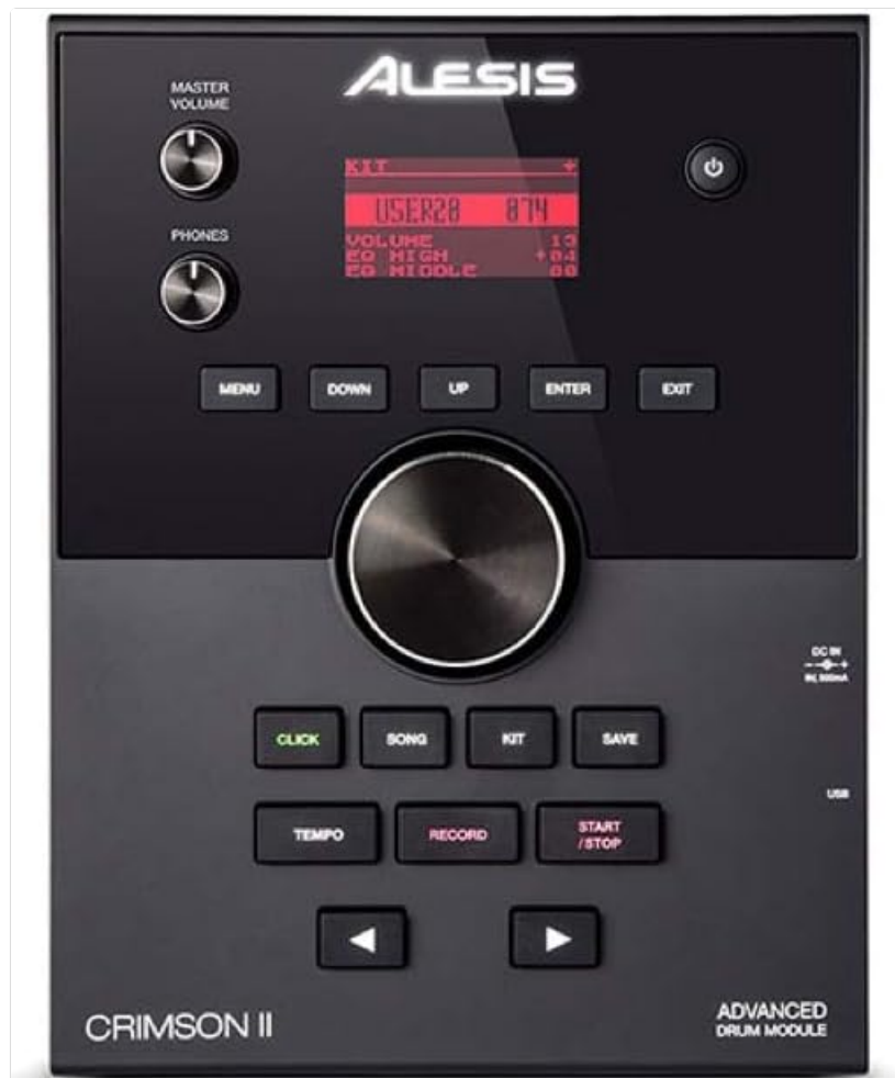
Figure 3: Front panel of the Crimson II module, displaying the main controls and LCD screen. This image shows the Master Volume, Phones volume, Menu, Navigation (Up, Down, Enter, Exit), Click, Song, Kit, Save, Tempo, Record, and Start/Stop buttons.
