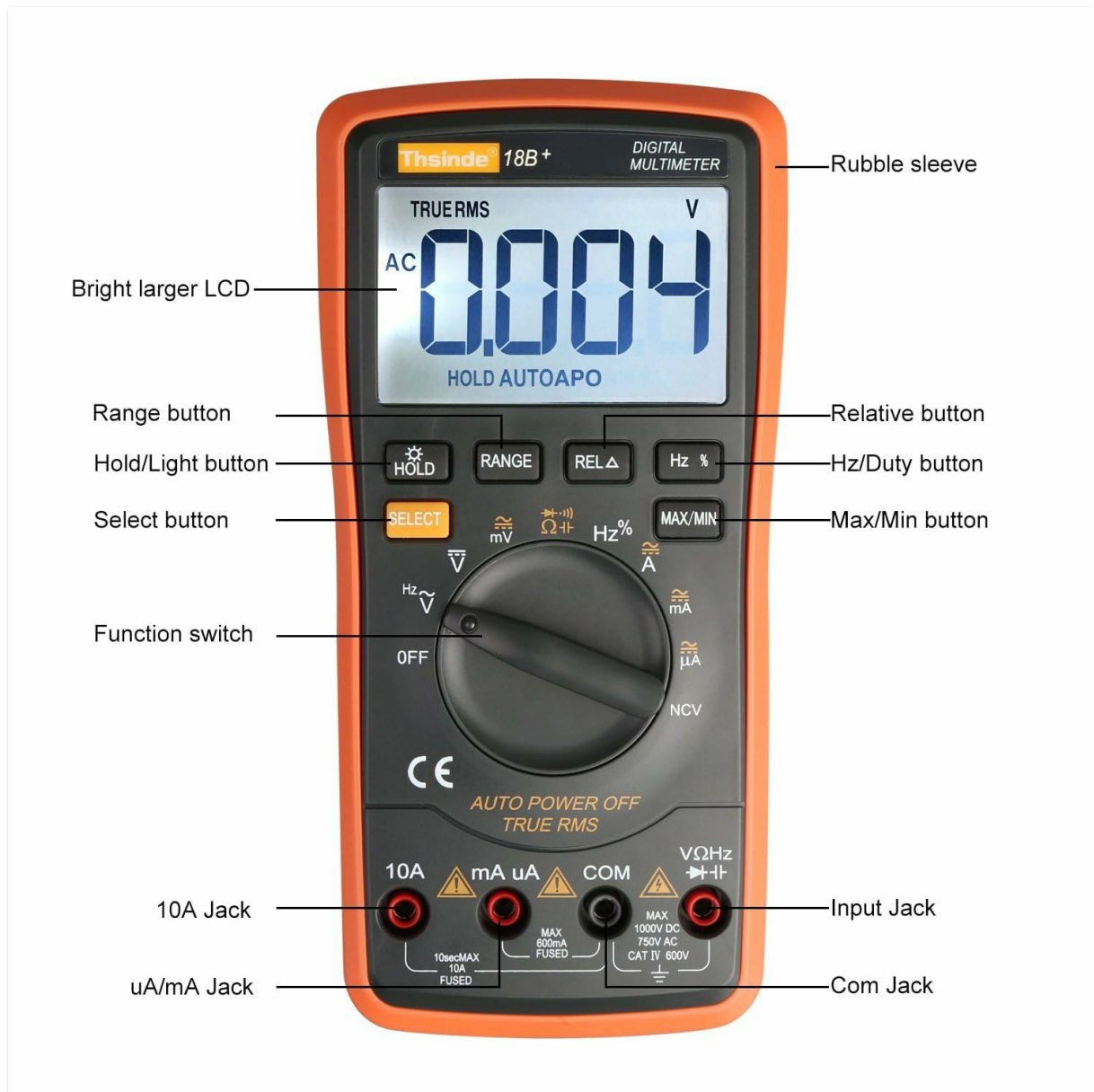
Figure 2.2: Multimeter Components Diagram
