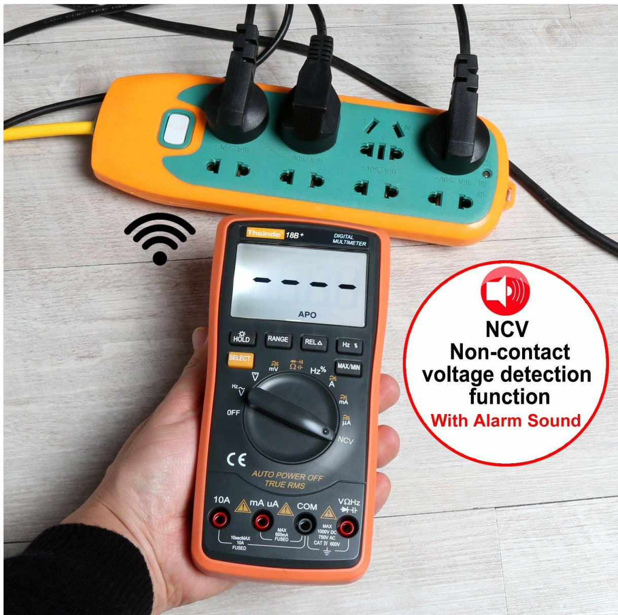
Figure 4.2: Non-Contact Voltage (NCV) Detection
